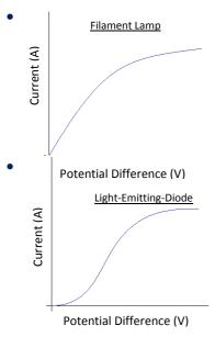
This is known as non ohmic; the current is not proportional to the potential difference. This is because the temperature changes as increased current passes through the filament. It is ohmic for small potential differences This is also non ohmic. For values of up to about 2 volts (depending on the colour of the L.E.D) the current remains at 0, so the resistance can be said to be infinite. Above 2 volts, the resistance decreases to allow current to pass through.
